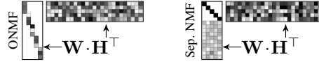
Figure 1: ONMF and Separable NMF, upon appropriate permutation of the rows of \mathbf{M} . In the first case, each row of \mathbf{M} is approximated by a single row of \mathbf{H}^\top , while in the second, by a nonnegative combination of all k rows of \mathbf{H}^\top .
